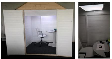
Figure 2. Cube design for lighting experiment and position of lighting instrument
